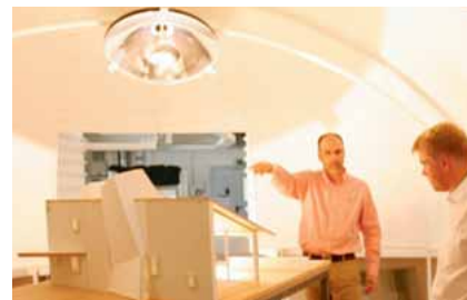
Left Physical model based lighting design simulation for a complex daylight environment in the artificial sky with sun simulator. (Source: Peter Andres, Lighting Consultant, Hamburg, Germany)
